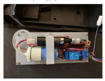
Connect the 4 PIN plug to the corresponding receptacle in the wiring harness:
