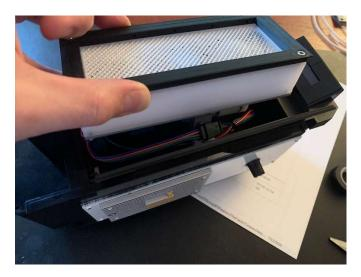
Begin to fit the smoke compartment into the trap ensuring no wires or hoses are caught around the edges. The harness will connect on the side shown, and will have just enough room to clear the side of the smoke add on kit.
