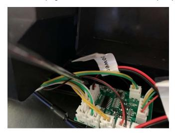
Connect the plug labeled "Green LED" to the port you disconnected the Green LED wiring from earlier.
