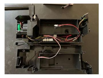
The harness should fit tightly through the hole originally occupied by a compartment LED.
